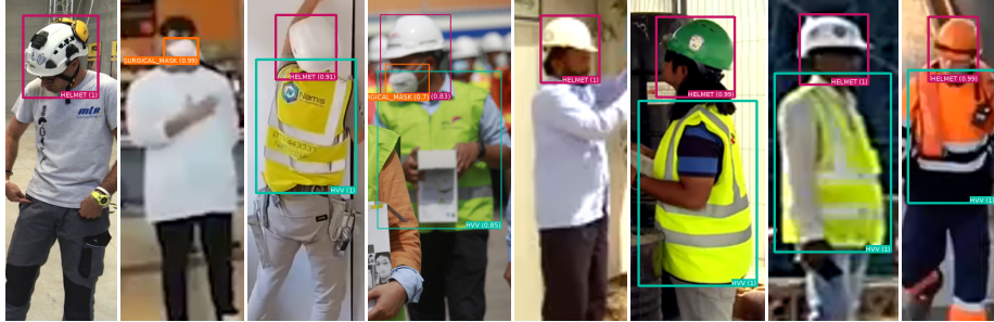
Figure 9: Examples of predictions of the PPE Detection module on our CrowdVisorPPE test set. PPE classes are color coded ( helmet , high-visibility vest , face mask ), and the detection score is reported in parenthesis.
