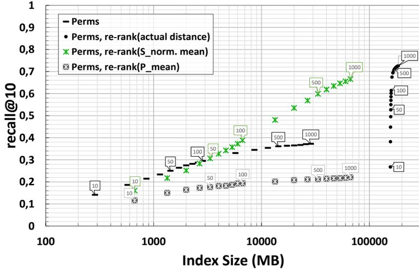
Figure 11: YFCC100M (10 million images subset), Euclidean distance:  $Recall@10$  as a function of the disk space used to store the index/features by various re-ranking techniques. For each approach that graph shows the results varying the prefix length  $l$  from 10 to 1000.
