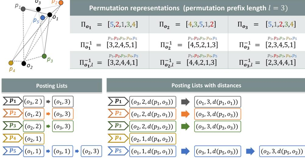
Figure 2: Examples of traditional posting lists and posting lists with distances, used to index three objects using five pivots and a prefix length  $l = 3$
