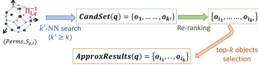
Figure 1: Illustration of the pipeline adopted in this work to compute the approximate  $k$ -NN results to a query by re-ranking a permutation-based candidate result set.
