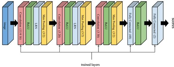
FIGURE 1: CNN ARCHITECTURE: FOR CONVOLUTIONAL LAYERS  $conv1-3$ , PARAMETERS ARE SPECIFIED AS “size/stride num”. FOR MAX-POOLING, PARAMETERS ARE SPECIFIED AS “size/stride”. FOR FULLY CONNECTED LAYERS WE REPORT THEIR DIMENSIONALITY. THE LAST FULLY CONNECTED LAYER IS FOLLOWED BY A 2-WAY SOFT-MAX CLASSIFIER.
