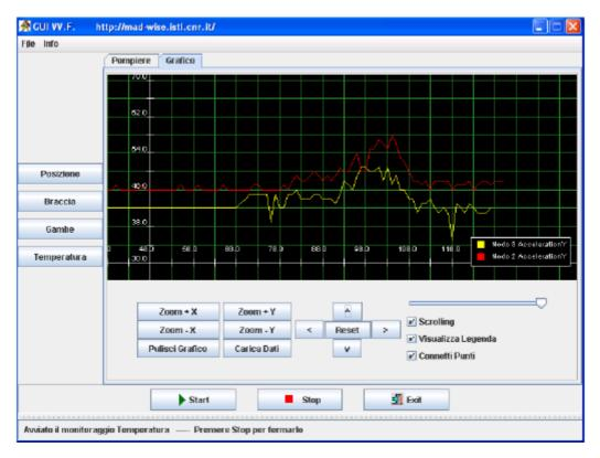
Figure 6. The graphical interface plotting the left arm movements.
